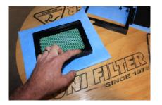
5. Unifiter recommends using sealing grease on the sealing edge of the air filter. (Bearing grease is the best option)
