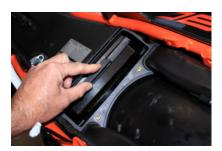
7. Install the air filter back into the bike and secure with the retaining wedge.
