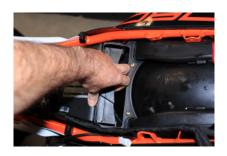
2. Remove air filter retaining wedge.
