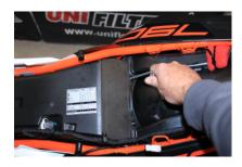
1. Remove air box access panel. (Wipe clean before removing)
