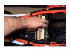
3. Remove air filter & air filter retaining box.
