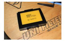
6. Place the air filter retaining box over the Unifilter.
