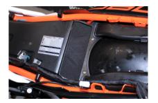
8. Place the black sealing foam on the top side of the filter. Unifilter recommends using the foam seal to prevent dust build up on the top sealing point.
